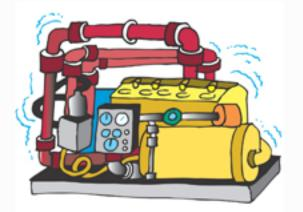
The biogas fuels the engine, which in turn spins an electric generator to create electricity. Waste heat from the engine is used to keep the digester warm, and offsets fuel purchases on the farm.
